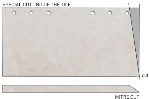
SPECIAL CUTTING OF THE TILE
